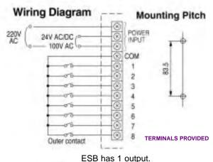
For panel mount application, cut square hole to 130mm. Panel thickness must be 5mm or less.
