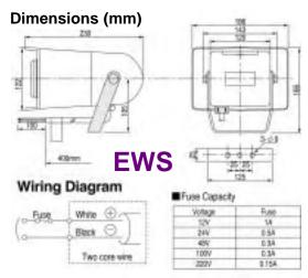
Sound selection is made by dip switch selection (Caution) polarity of power supply in case of DC
