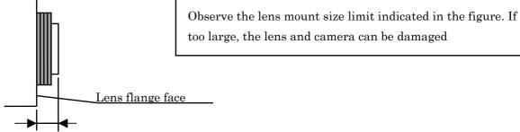
T: HV-D27A: Less than 3.8 mm HV-D37A: Less than 4.3 mm
