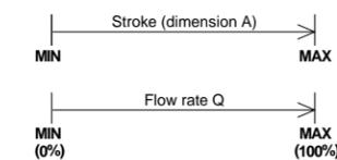
Adjust the stroke by turning the adjustment rod to control flow rate when the valve is open.
