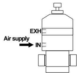
Single action is standard for the FV-5000 · FV-7000 Series. The valve closes when operating air is cut off.
