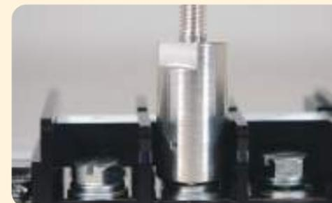
The butt contact is used in the current test of a general-use terminal board. Even more stable energization is ensured by energizing the two directions of the upper and lateral sides using two coil springs for the screw head. Designing and manufacturing custom-made products are accepted in accordance with the size of the screw head of the terminal board.
