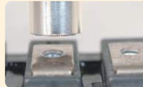
The butt contact is used in the current and breakdown tests of the pre-shipment inspection of the IGBT. Stable energization is ensured by multipoint contact, and damage to the terminal block of the IGBT can be minimized. Large deflection, which is one of the key features of a coil spring, compensates for any misalignment in the direction of height when more than one terminal is energized at the same time.
