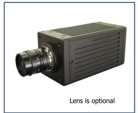
The used sensor is VGA resolution, 20 micron pixel size and has the sensitivity from 950nm to 1700nm. The interface is Camera Link or Gigabit Ethernet (1000BASE-T). .Lens mount is conventional C mount and lenses of more than 1-inch format should be used. Bluevision SWIR series lenses, 20mm, 24mm, 28mm, 35mm, 50mm and 105mm lenses C mount type are available.
